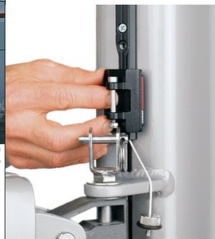
Cars are easily removed from the track by freeing the screwpin endstop and sliding them off.
